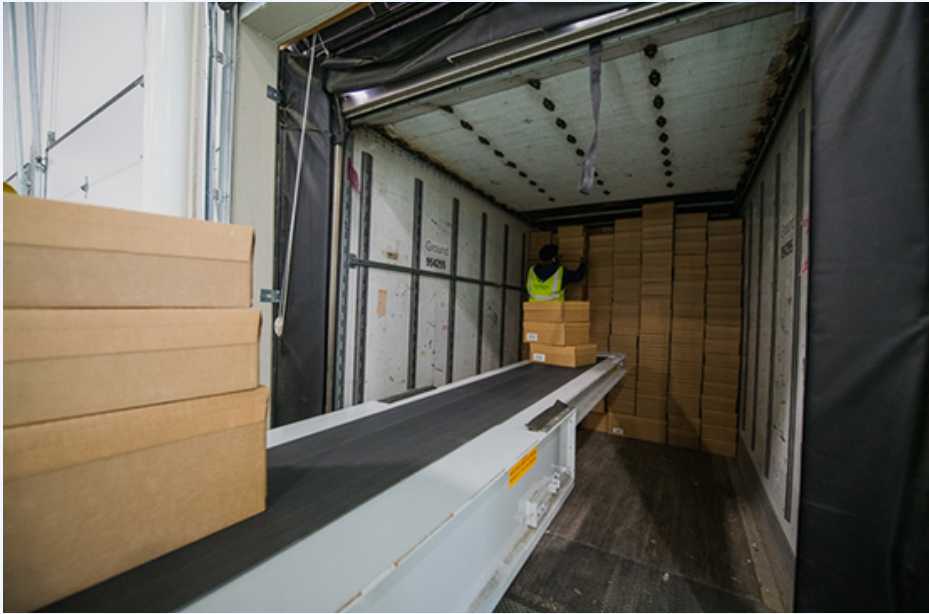
Image of an unloading Adjustoveyor in use
